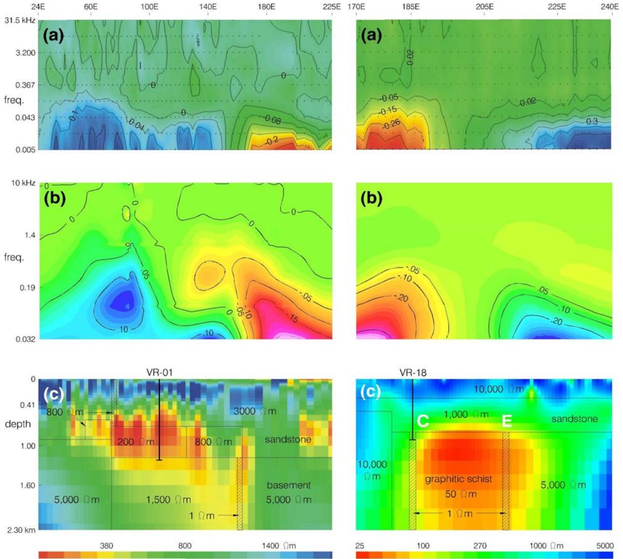
Figure 2: Stewardson Lake AMT survey. Imaginary part of (a) observed and (b) modeled TE mode tipper. (c) Imaged resistivity from 2 D inversion and forward model with basement conductor.
