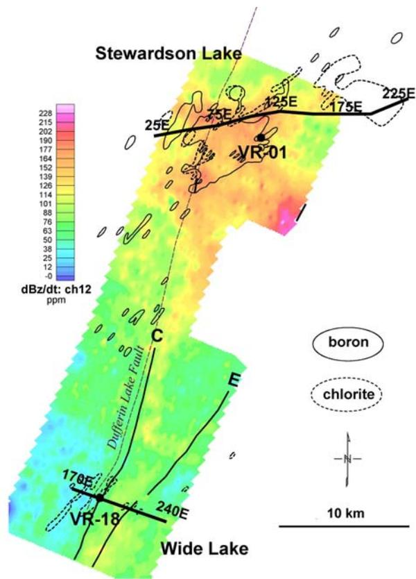
Figure 1: Sandstone alteration, conductors, drill holes and AMT profiles in the Virgin River study area. Image plots the channel 12 amplitude of the GEOTEM vertical magnetic induction. Note the high amplitudes (conductivity) at Stewardson Lake.
